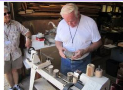
**July Lathe Turning SIG** demonstrated the use of various work holding chucks and jaws. He had what are known as Cole jaws for holding the edge of a bowl. Ed then made a jam chuck for his bowl using stacked pieces of MDF. He also made a jam chuck for holding a turned egg. Finally, a collet chuck was used to turn a bottle stopper.
