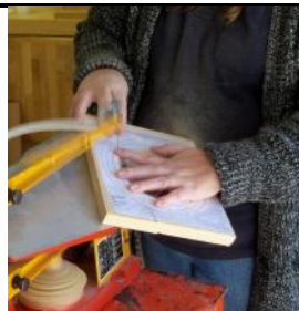
March Scroll Saw SIG was held at Bob Beckert's shop where the gang tried their hand at making scroll saw bowls. This involves tilting the table to 28°, cutting concentric circles and then gluing then the circles together. It is harder than it looks!
