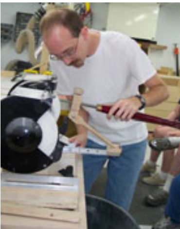
Jason Beam demonstrated his own jig to enable him to apply a finger nail grind to his spindle gouge.
