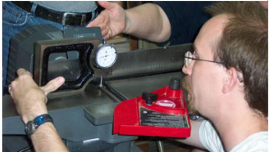
Jason uses his Oneway to allow him to accurately position the blade to the plane of the out feed table of the jointer.
